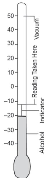
Figure 8.2 Minimum Thermometer
