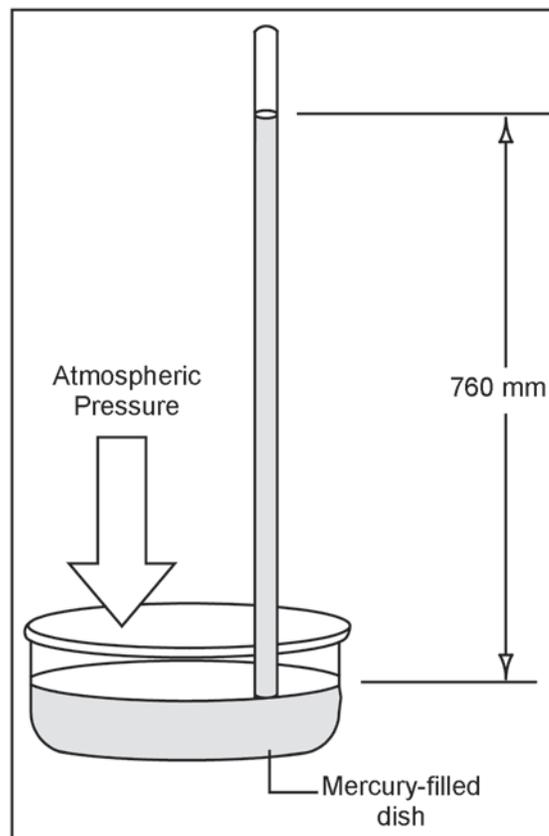
Figure 8.4 Mercury Barometer
