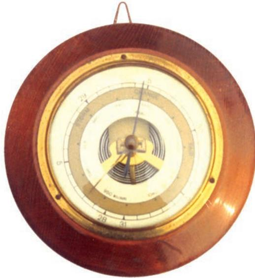
Figure 8.5 Aneroid Barometer
